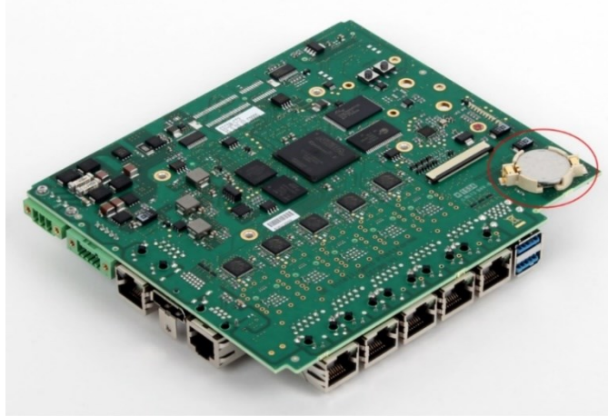
Figure 7: Location of RTC Battery on CPE400/CPL410/CPS400
